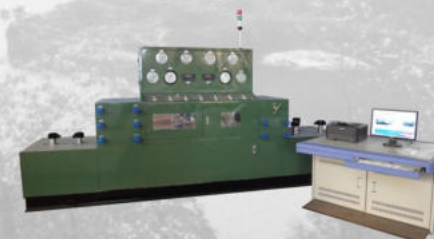
YFS-A100/300型 智能型液压安全阀试验台 (套式) Intelligent Type Hydraulic Safety Valve Test Bench of Model YFS-A100/300(Combined Type)
