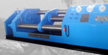
PZ-600t型 阀门压力测试机 Valve Pressure Testing Machine of Model PZ-600t
