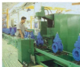
YFS-DX型 液压低压闸阀试验台 (自动线) Hydraulic Low Pressure Gate Valve Test Bench of Model YFS-DX (Automatic Production Line)
