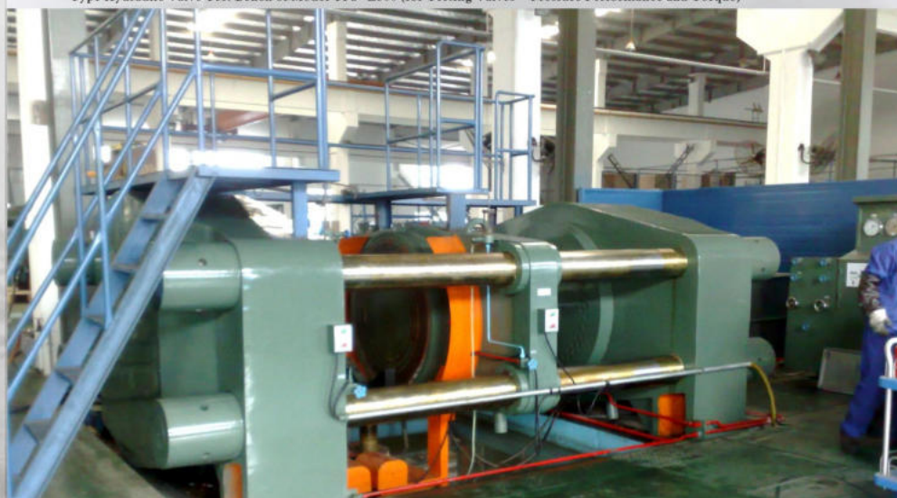
使用单位: 伟尔格普流体控制(苏州)有限公司 User: Weir Valves and Controls (Suzhou) Co., Ltd. 设备型号: YFS-D2200t型 液压阀门试验台 (用于试压大口径、高磅级球阀、抽气截止阀等) Machine Model & Description: Hydraulic Valve Test Bench of Model YFS-D2200t (for Testing Large Size and High Pressure Ball Valves, Extraction Check Valves etc.)
