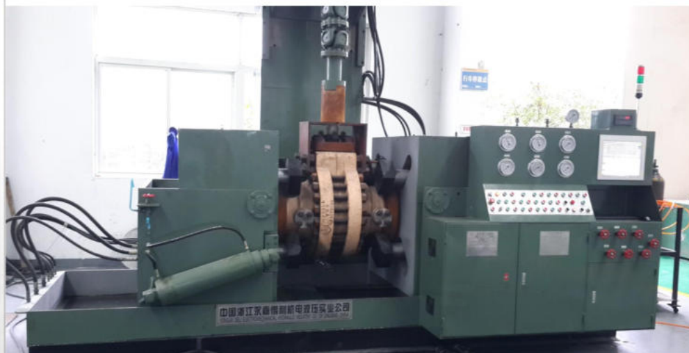
使用单位: 江苏神通阀门有限公司 User: Jiangsu Shentong Valve Co., Ltd. 设备型号: YFS-Z500型智能型液压阀门试验台 (用于阀门压力性能测试和扭矩测试) Machine Model & Description: Intelligent Type Hydraulic Valve Test Bench of Model YFS-Z500 (for Testing Valves' Pressure Performance and Torque)
