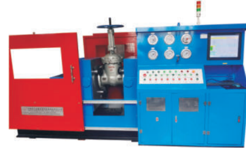
YFS-Z型 液压阀门试验台 适用于试压DN15-1200, 150-2500LB 法兰式阀门 (闸、球、截止、止回阀等), 可选配电脑PLC系统。 Hydraulic Valve Test Bench of Model YFS-Z Series: Suitable for testing flange end valves (gate, ball, globe, check valves etc.) with nominal size range DN15-1200 and nominal pressure range 150-2500LB, can be equipped with computer PLC system for option.
