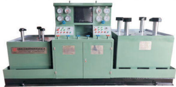
YFS-DL型 液压阀门试验台 适用于试压DN50-3000, 150-2500LB 蝶阀和对夹式止回阀, 可选配电脑PLC系统。 Hydraulic Butterfly Valve Test Bench of Model YFS-DL Series: Suitable for testing butterfly valves or wafer type check valves with nominal size range DN50-3000 and nominal pressure range 150-2500LB, can be equipped with computer PLC system for option.
