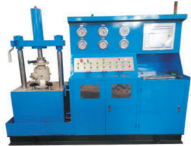
YFS-L型 液压阀门试验台 适用于试压DN15-400, 150-4500LB 法兰式、焊接式和螺纹式阀门 (闸、球、截止、止回阀等), 可选配电脑PLC系统。 Hydraulic Valve Test Bench of Model YFS-L Series: Suitable for testing flange, weld and thread end valves (gate, ball, globe, check valves etc.) with nominal size range DN15-400 and nominal pressure range 150-4500LB, can be equipped with computer PLC system for option.
