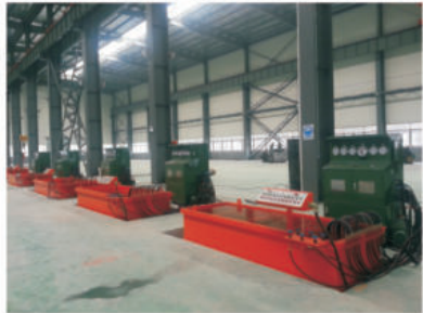
YFS-ZC型 卧式液压阀门试验台 适用于试压DN15-1000, 150-2500LB 法兰式阀门 (闸、球、截止、止回阀等), 可选配电脑PLC系统。 Hydraulic Valve Test Bench of Model YFS-ZC Series (Submerged type): Suitable for testing flange end valves (gate, ball, globe, check valves etc.) with nominal size range DN15-1000 and nominal pressure range 150-2500LB, can be equipped with computer PLC system for option.
