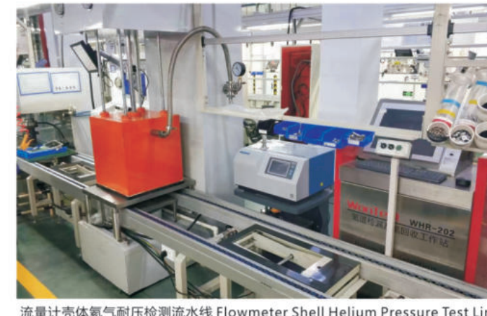
流量计壳体耐气压检测流水线 Flowmeter Shell Helium Pressure Test Line
