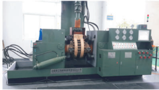
YFS-ZN型 智能型液压阀门压力/扭矩试验台 适用于试压DN15-1200, 150-2500LB 阀门压力性能试验 (50-50000N.M) 阀门启闭扭矩试验 Hydraulic Valve Test Bench of Model YFS-ZN Series (Intelligent type): Suitable for DN15-1200, 150-2500LB valve pressure test and 50-50000N.M valve open-close torque test.
