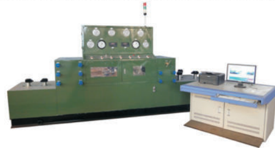
YFS-A型 液压安全阀试验台 适用于试压DN15-400, 150-2500LB 安全阀, 可选配电脑PLC系统。 Hydraulic Safety Valve Test Bench of Model YFS-A Series: Suitable for testing safety valves with nominal size range DN15-400 and nominal pressure range 150-2500LB, can be equipped with computer PLC system for option.
