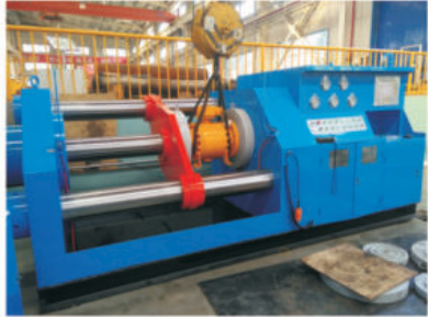
YFS-D型 液压阀门试验台 适用于试压DN15-1800, 150-4500LB 法兰式和焊接式阀门 (闸、球、截止、止回阀等), 可选配电脑PLC系统。 Hydraulic Valve Test Bench of Model YFS-D Series: Suitable for testing flange and weld end valves (gate, ball, globe, check valves etc.) with nominal size range DN15-1800 and nominal pressure range 150-4500LB, can be equipped with computer PLC system for option.
