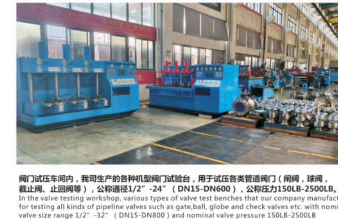
YFS-D1200型 液压阀门试验台 (大型智能型), 最大试压到48" ( DN1200 ) -600LB 管线阀门 ( 球阀, 闸阀, 截止阀, 止回阀等 ), 最高水压120MPa, 设计最大承受力2800吨 Hydraulic Valve Test Bench of Model YFS-D1200(Big and intelligent type), for testing pipeline valves such as ball, gate, globe and check valves etc. with max. valve size up to 48" ( DN1200 ) - 600LB, max. test water pressure 120MPa, designed max. bearing(reaction) force 2800 Tons.
